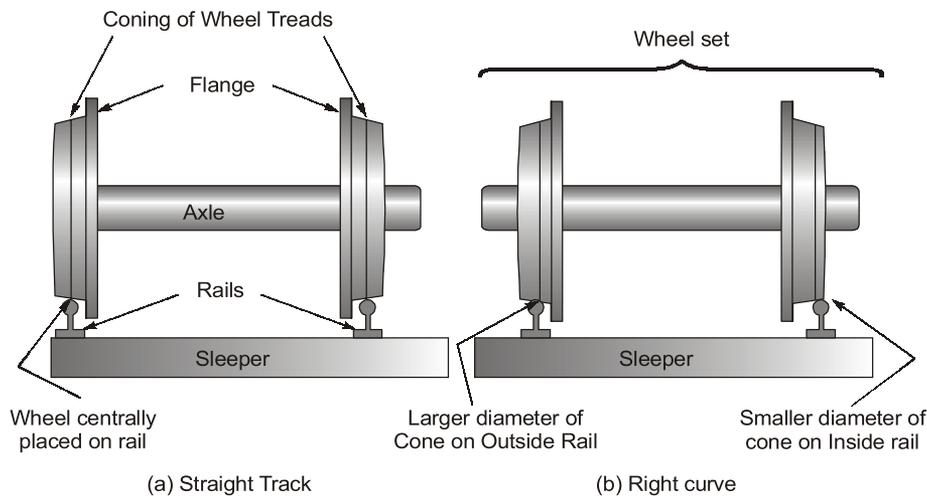
Fig. Coning of Wheels
