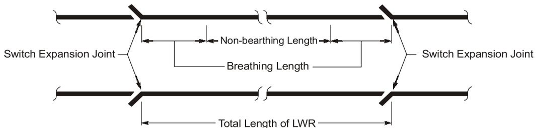
**Fig. Long Welded Rail**
