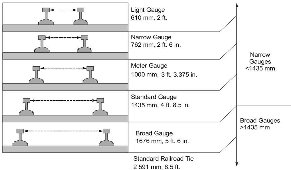
Fig. Gauges of Railway Track
