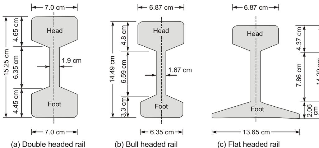
Fig. Types of Rail Sections
